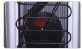
Hermetically sealed reciprocating Compressor
