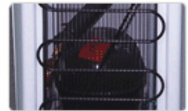
Hermetically sealed reciprocating Compressor
